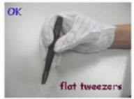
8. Please do not bend the film near the substrate glass. It could cause film peeling and TAB/FPC/COF damage. For TAB, It should bend the slit area as actual OLED it is. For FPC or COF, it is suggested to follow below pictures for instruction (distance between substrate glass and bending area >1.5mm; R>0.5mm).
