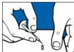
2. Insert tip of RIT tool into the top of the receptacle and, with slight hand pressure, seat the receptacle into the drill hole until resistance is met.
