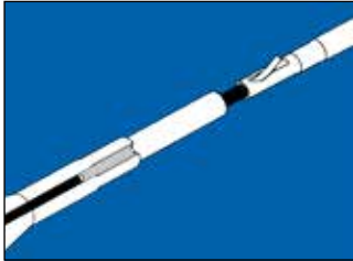
3. Hold wire firmly against tool with forefinger. Insert protruding wire into termination end of W-4 receptacle. Release grasp on wire and push insulator onto end of receptacle, completing termination.
