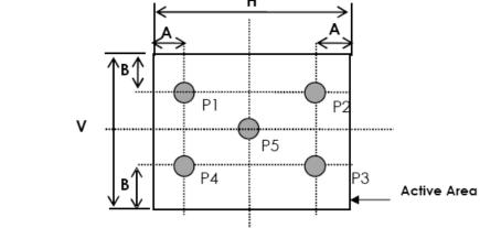
Light spot size  $\emptyset$ =7mm, 500mm distance from the LCD surfade to detector lens measurement instrument is TOPCON's luminance meter BM-5
