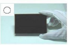
As above photo, please handle with anti-static gloves around LCD edges.
