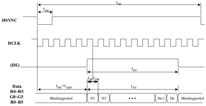
Remark : If SYNC mode is used, please fix DE signal to low, DE timing waveform is for reference only.
