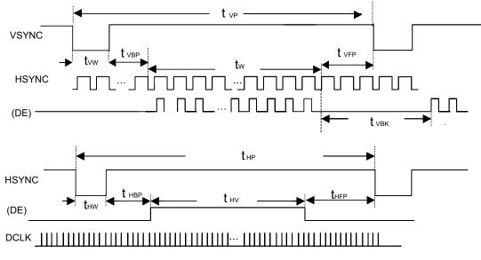
Remark : If SYNC mode is used, please fix DE signal to low, DE timing waveform is for reference only.
